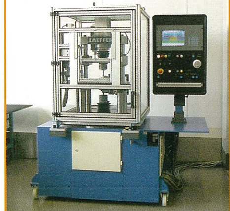
SPM 12: Testing press to compact green radioactive material samples.
